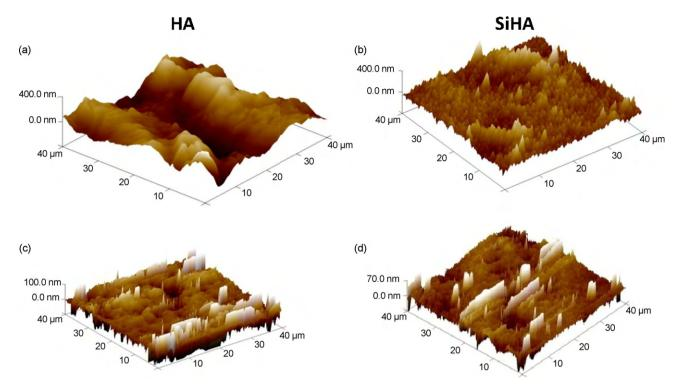
Fig. 2. AFM images of original (a) HA and (b) SiHA surfaces and of polished (c) HA and (d) SiHA surfaces.
