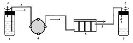
**Fig. 1.** Schematic diagram of the bioreactor system placed in the constant temperature oven (37 °C). A silicone tube (3) makes the connection between fresh medium bottle (1), which supports an air filter (2), bioreactor (5) and waste medium bottle (6). A multi-channel peristaltic pump (4) placed just before the bioreactor is adjusted to a constant flow fluid at 2 mL/h.
