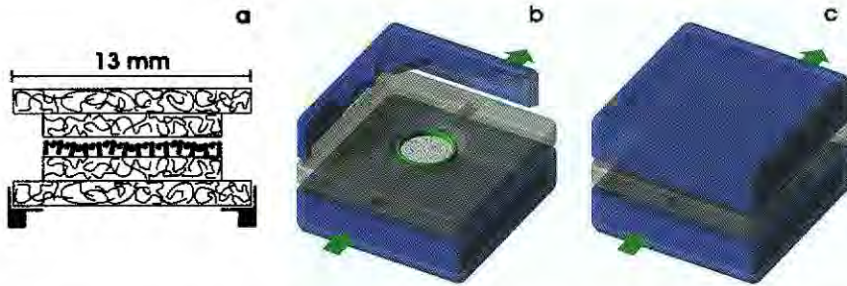
Fig. 7 Microreactor design for the culture of a basic sandwich set-up at the interface of an artificial interstitium. (a) The basic sandwich set-up containing renal stem/progenitor cells is mounted in a tissue carrier. (b) The perfusion container consists of a base plate to hold the tissue carrier with the developing tissue embedded between layers of polyester fleece. (c) The container is sealed for culture with a lid
