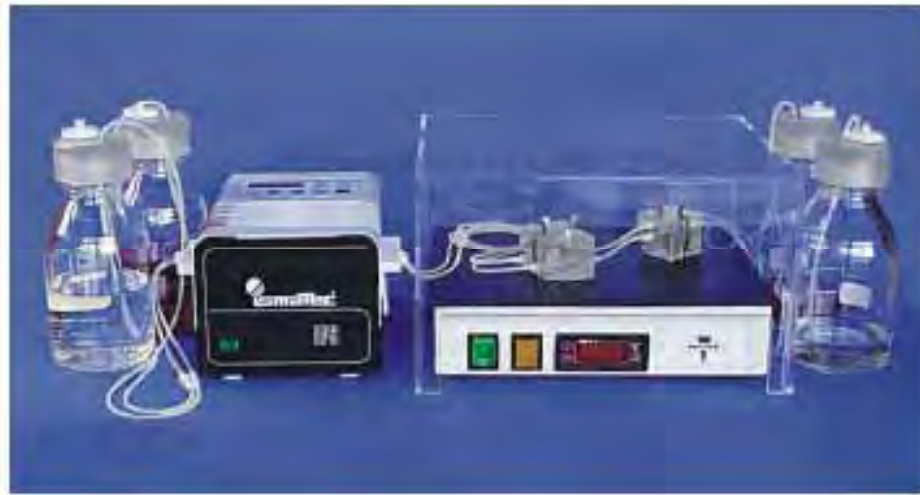
Fig. (5). Gradient perfusion culture is performed on a laboratory table. A peristaltic pump (left side) transports the media (1 ml/h) from the storage bottles to a gas expander module and onward to a gradient container. The waste medium is collected in the bottles on the right side. A heating plate and a lid maintain the desired temperature.
