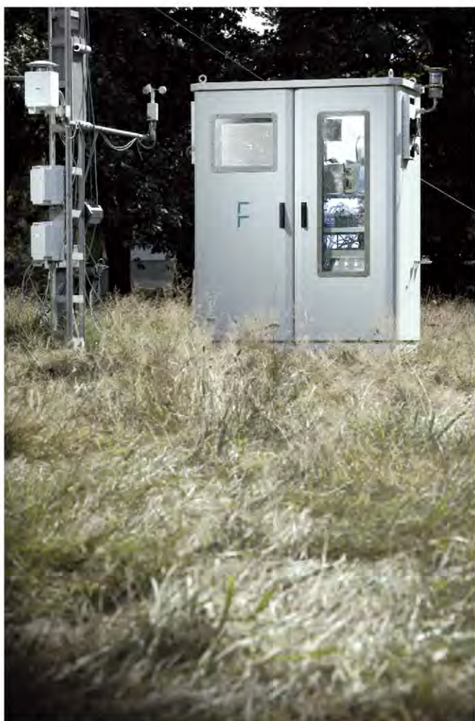
Fig. 4 The Karlsruhe exposure system for lung cells in outdoor conditions.
