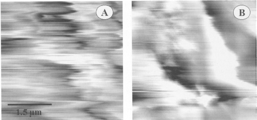
Fig. 11.7 Scanning lateral force microscopy. (A) Min3-modified surface; the streaks indicate a strong adhesion during the visualization of the surface; (B) the same surface area was scanned, but the interaction was blocked by soluble Min3.
