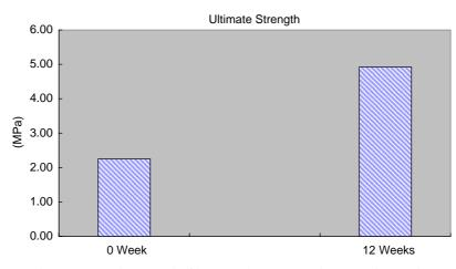
Fig. 7. Compressive strength of beta-TCP/BMO composite at 0 and 12 weeks.
