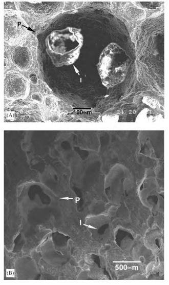
Fig. 4. SEM photomicrograph of microstructures of the novel porous hydroxyapatite (A) and beta-TCP(B). P indicates pore and I indicates interconnecting path.
