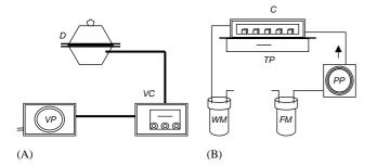
Fig. 3. Schematic diagram of the low-pressure system (A) and perfusion culture system (B). In (A), D stands for polycarbonate vacuum dessicator, and  $V_c$  for vacuum controller; in (B), C stands for perfusion container, TP for thermoplate, PP for peristaltic pump, FM for fresh medium, and WM for waste medium.
