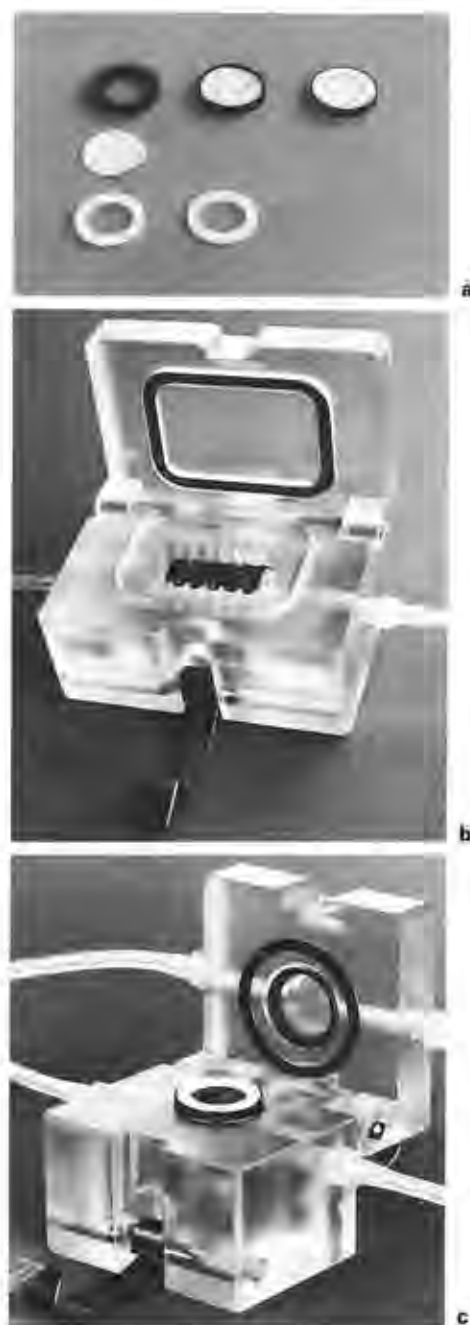
Fig. 3a-c. Kidney-like culture conditions. a The cells are grown on a special holder set with individually exchangeable supports. b, c In the newly developed cell culture containers the cultures are continuously supplied with fresh medium. In the perfusion container ( b ) the cell holder sets are bathed with the same culture medium on both the top and the bottom. In the gradient perfusion container ( c ), however, the cells are supplied with completely different media from above and below, just like in the actual kidney.
