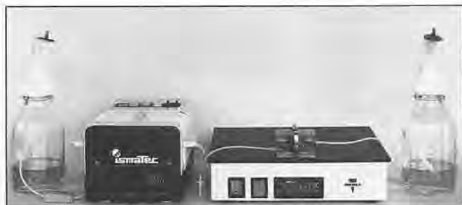
Figure 3. The perfusion culture system runs on a laboratory table. The medium is transported with a peristaltic pump with 1 mL/h from the left bottle into the container on the warming plate (37°C). The waste medium is collected in the bottle at the right side. Because pH-stabilized media are used, the system works outside an incubator for weeks and months.
