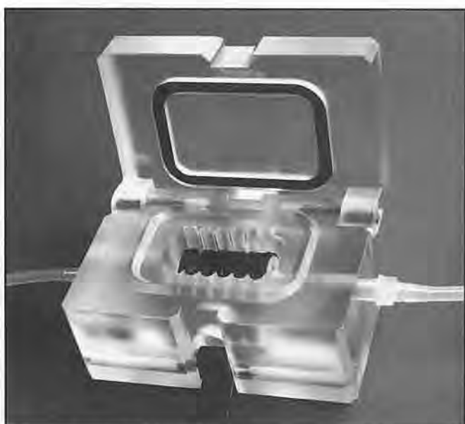
Figure 2. Perfusion culture container. After adherence of cells on the support, the cell carriers are transferred, using a fine forceps, to a newly constructed perfusion culture container. Medium is pumped in at the left side, crosses between the cell carriers and leaves at the right side.
