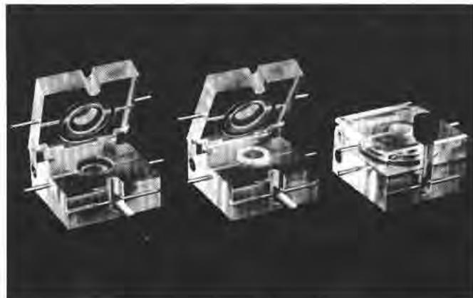
Fig. 5. Photographic illustration of mounting a MINUSHEET in the gradient superfusion chamber: left side—open chamber, middle—positioning of a sheet into the chamber and right side—closing of the chamber by fastening the frontal lever screw. The specific construction makes it possible to culture cells under a luminal-basal medium gradient. Single sheets with the mounted epithelium are easily placed by a pair of forceps in the gradient superfusion chamber. Iso-, hypo- or hypertonic media can be used either at the apical or basal side of the epithelium through the inlet and outlet cannulas in the lid and base.
