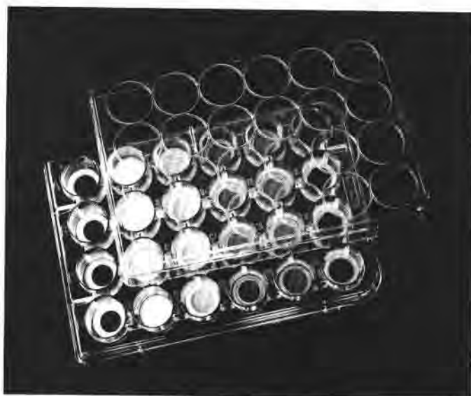
Fig. 2. Photograph of a 24-multiwell tissue culture plate with mounted cell holder sets. The figure depicts the wide versatility of cell holder sets which can be discerned from six different interchangeable support materials marked by different color codes. The cell holder sets are used to improve the attachment characteristics of the plastic culture dish.
